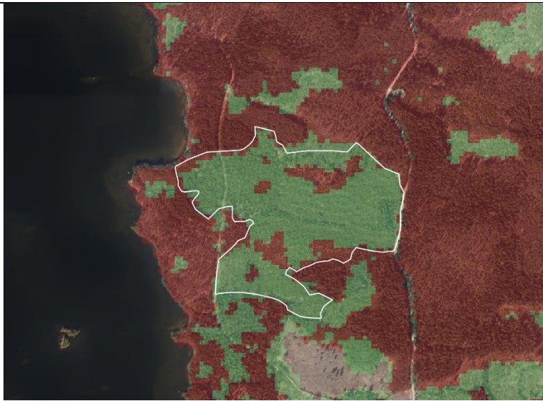
Fig. 3: Spruce-dominated young growing forest partly misclassified as broadleaved (green) in HRL DLT. Stand is delineated with white polygon.
