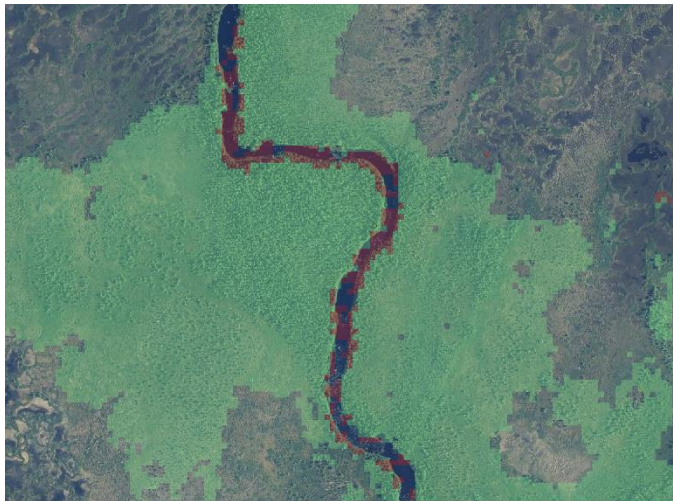
Fig. 4. Commission error on coniferous. HRL DLT overlaid over aerial imagery. River and broad-leaved (birch) trees classified as coniferous (red). Surrounding area is correctly classified broad-leaved (green).
